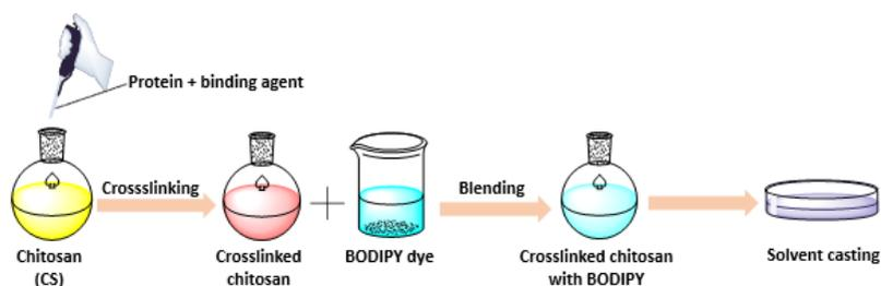
Fig. 4. Preparation of protein-crosslinked chitosan films with BODIPY.
