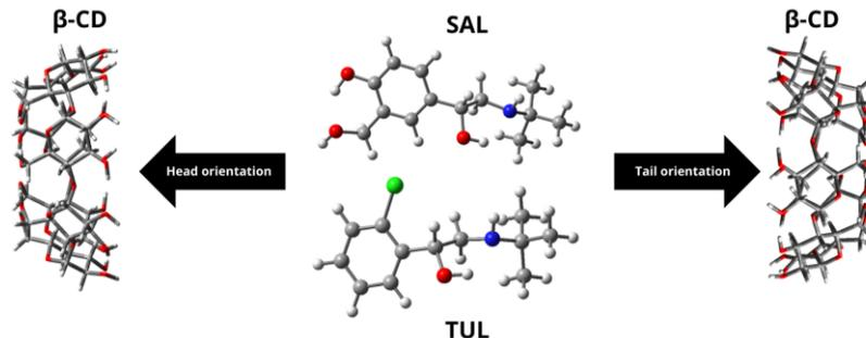
Fig. 1. Orientations of drug molecules inside  $\beta$ -cyclodextrin
