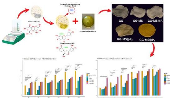
Fig. 1. Synthesis and fabrication of Sponges based on Gellan gum/*Musa sapientum*/*Cucurbita maxima* with their antioxidant and anti-inflammatory activity
