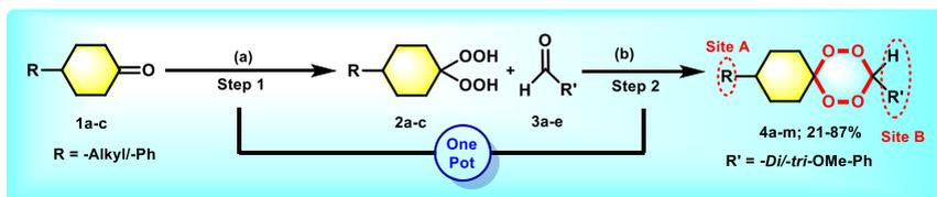
**Fig. 1.** Classical two-step one-pot approach for functionalised mono-spiro-1,2,4,5-tetraoxanes (**4a-m**) syntheses.
